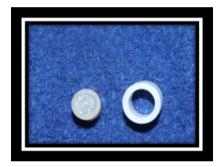
*Figure 1b:* 6mm x 6mm Cylinders with everX Posterior core (4 mm) and Solare X overlay bonded to dentin disks.
