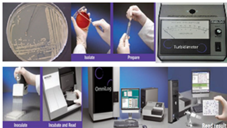
Figure 1: BiOLOG Micro Station identification steps and whole set equipment.
